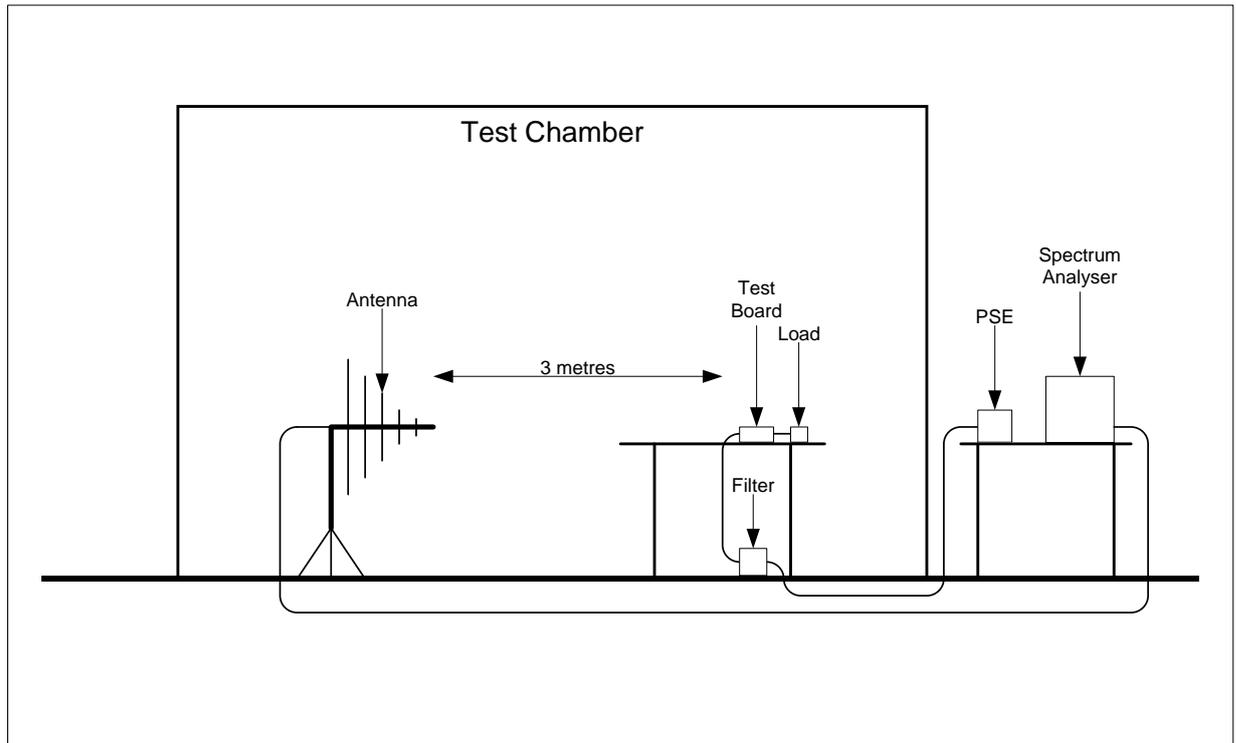
**Figure 1: Test Setup – Emissions**
