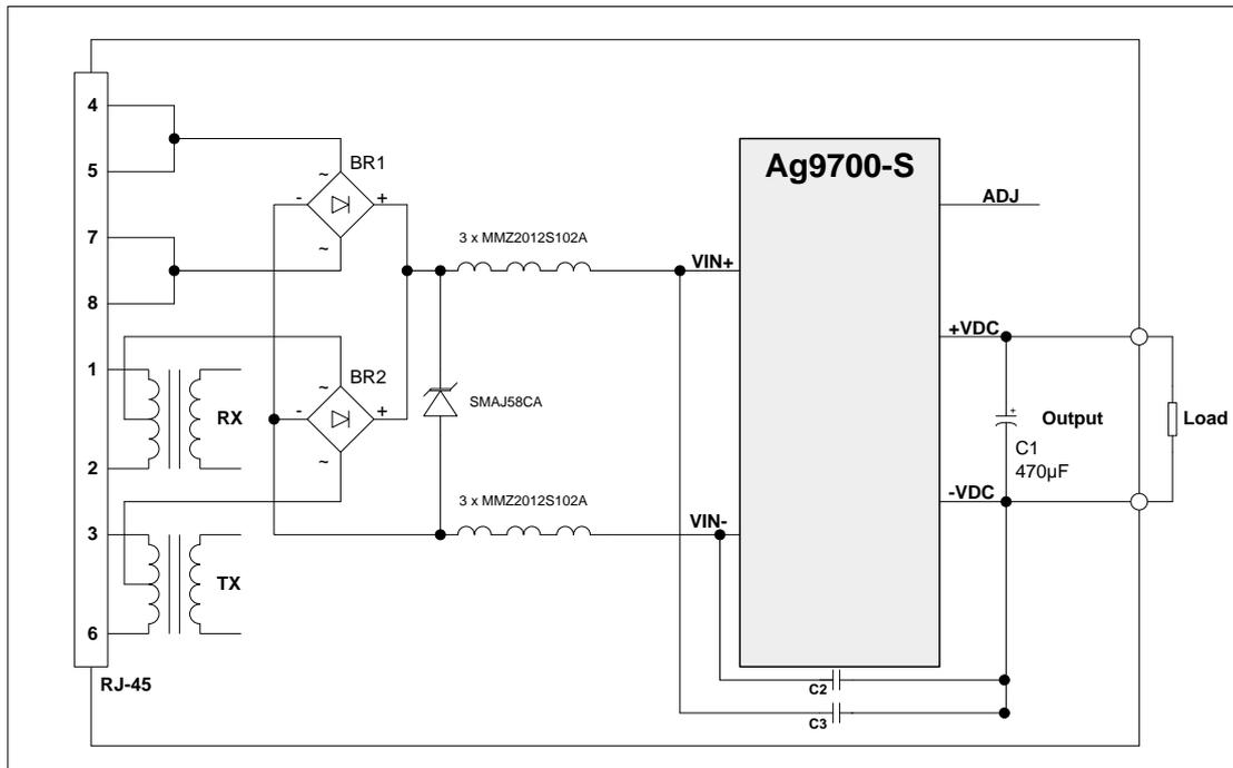
Figure 4: Chip Bead and 'V' Capacitor Filter for -S
