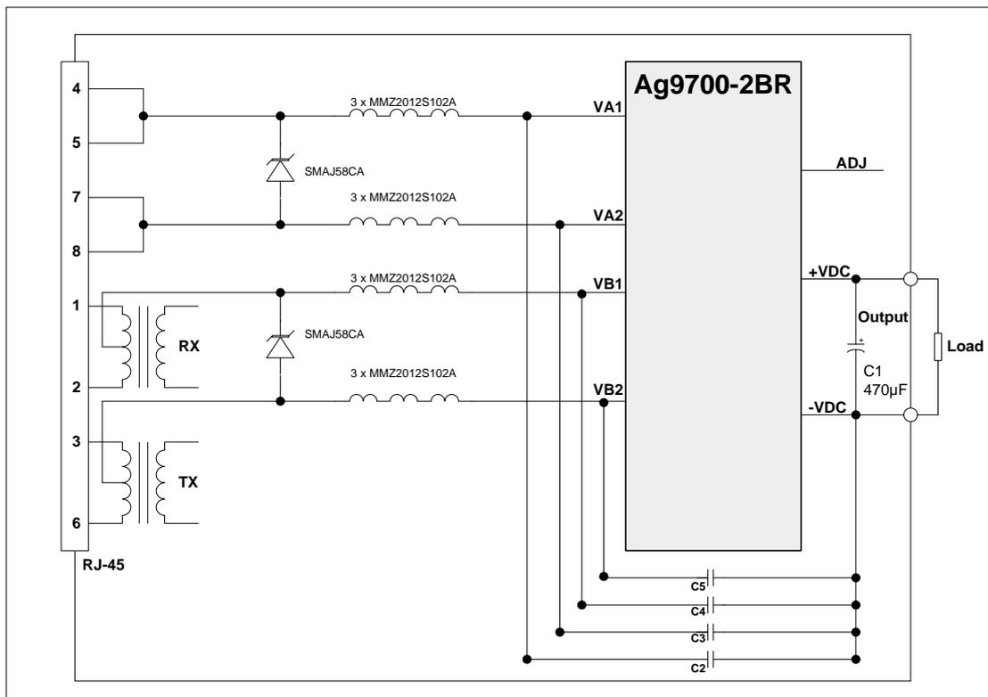
Figure 5: Chip Bead and 'V' Capacitor Filter for -2BR or -FL
