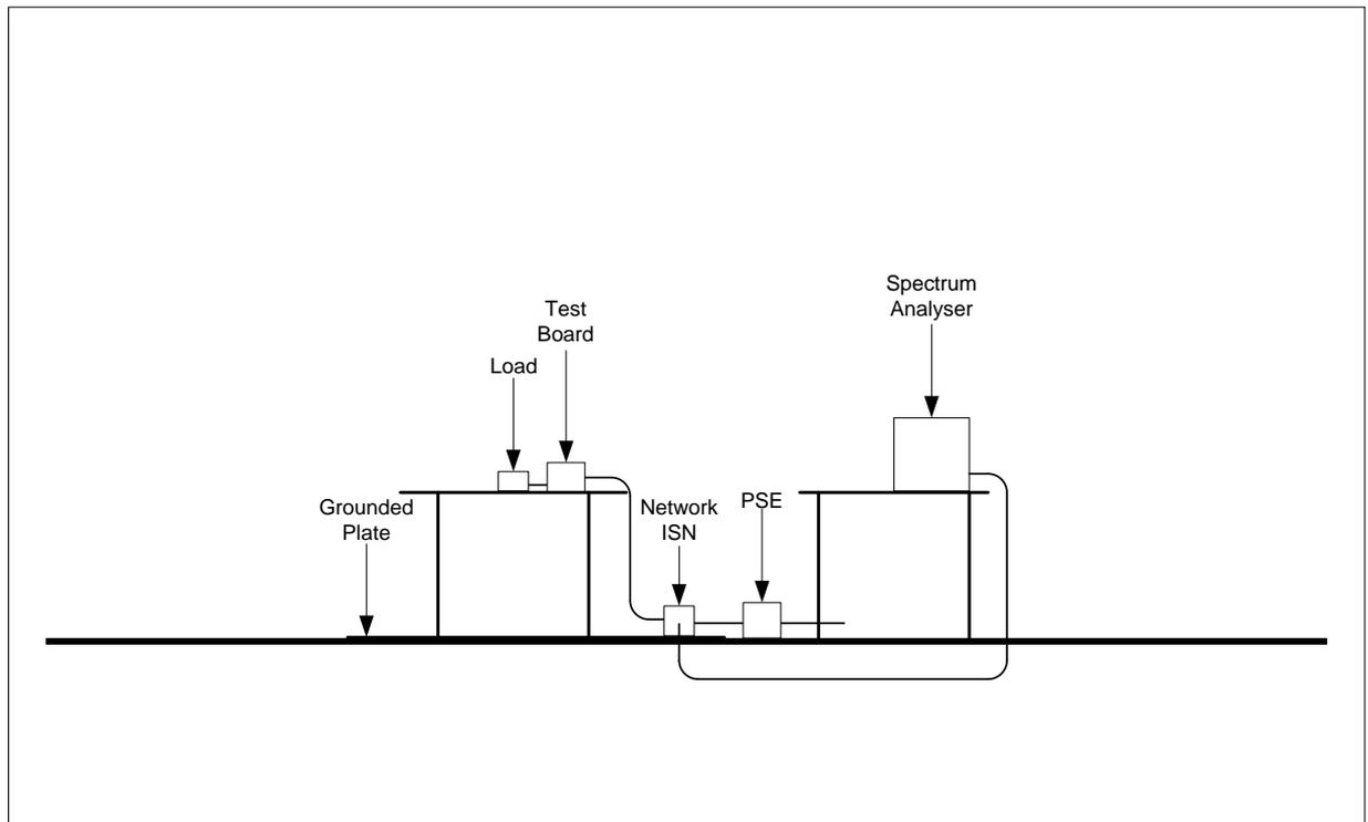
**Figure 2: Test Setup – Conducted**
