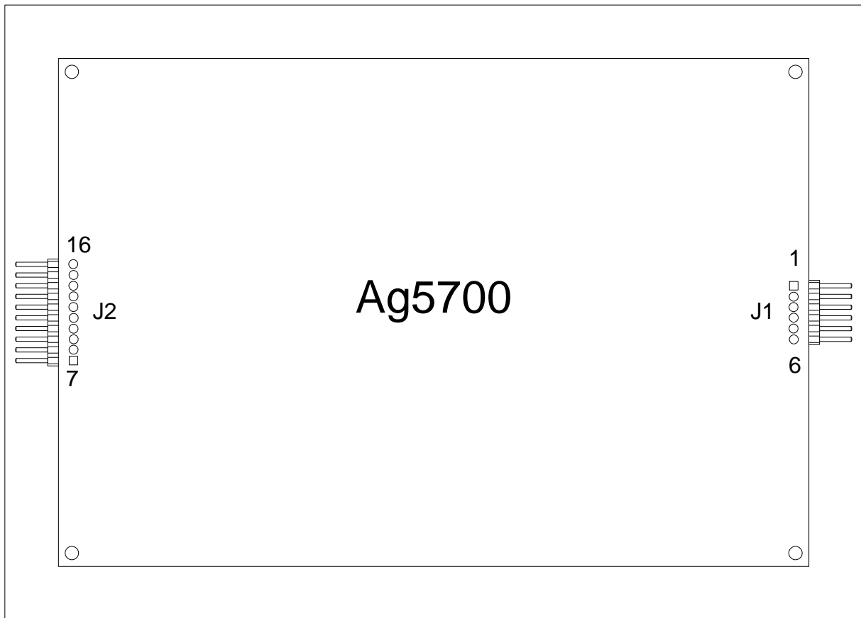
Figure 2: Ag5700 Package Format
