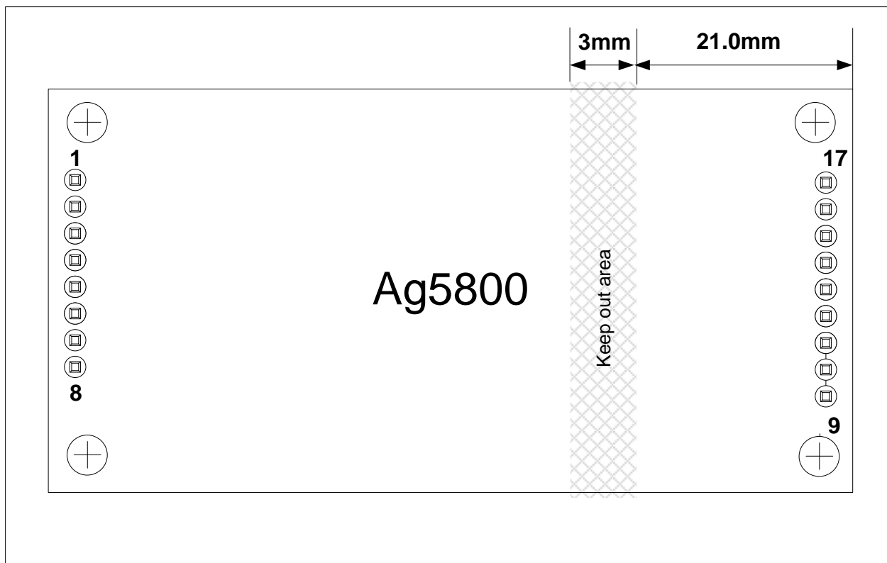
Figure 17: Position of the Isolation Barrier
